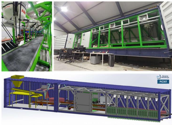
PICKIT Lab and Pilot Scale : Mobile prototype for single pass-multiclass robotic sorting of scraps
